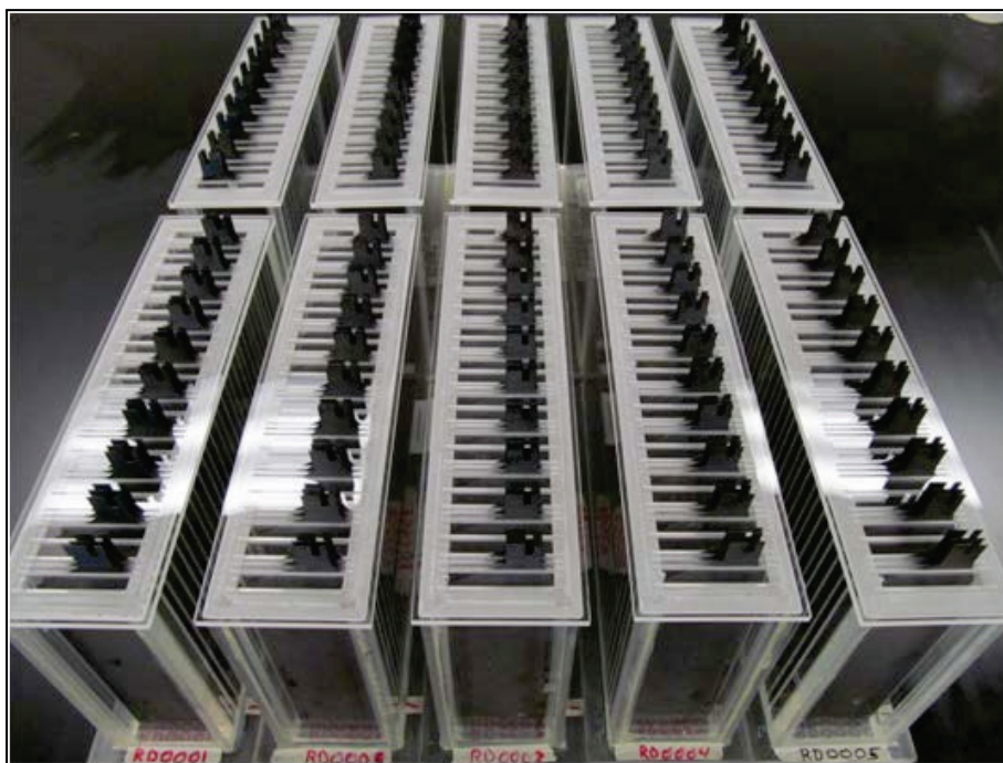
Figure 39. 1-kW Zinc-air Prototype (Photo courtesy of EOS Energy Storage)
